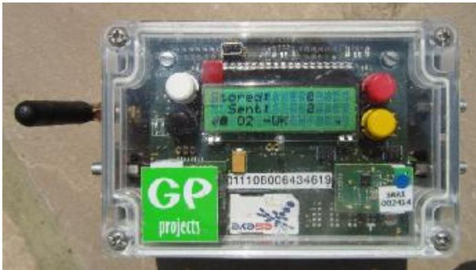
Punch data transmitted by an Eider unit is sent to the GPProjects servers, where it is stored ready for viewing. The data can either feed an online view of race data, or be pulled into a commentary software such as AutoDownload or Mercs by the Retriever software.
