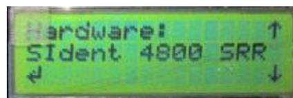
This menu selects what hardware is connected to device. SPORTident operates at either 4800 or 34000 baud rate. Therefore the options are:
