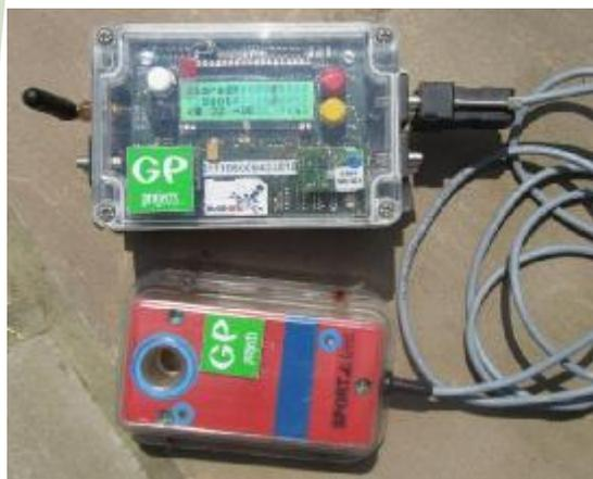
The Eider system provides a method of delivering punch data from remote controls wirelessly for safety or commentary purposes. Using the mobile phone networks (GPRS data), the Eider Control sends race data directly to the internet, from where it can be viewed for live web results, or pulled into commentary software. Short Range Radio (SRR) and merge modules give the Eider Control increased flexibility.
