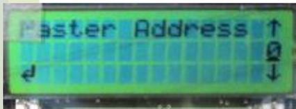
The master address identifies where Kestrel Controls send their punch and status data. Set the number to the node address of the receiving Master Kestrel unit. Conventionally this is '0'. Note: there should only be 1 Master Kestrel unit on a radio frequency channel.
