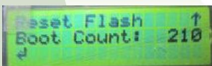
The boot count is the number of times the flash memory in unit has been reset, and helps in time correction by setting a 'baseline'. This should not need to be changed. However, if you need to reset the flash, press the white button on this menu. This will reset the 'Sent' counter to zero and return you to the previous screen for confirmation.
