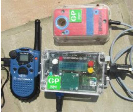
The Kestrel system provides a method of delivering punch data from remote controls wirelessly for safety or commentary purposes. Using FSK radio technology, the Kestrel Control unit sends race data to a receiving Master Kestrel unit connected to a computer running event software. Short Range Radio (SRR) and Merge modules enable greater flexibility and functionality of the Kestrel Control.
