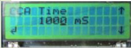
The Clear Channel Assessment (CCA) time defines how long the radio module listens on the channel to see if someone else is using it before transmitting data. Logically, this should be longer than key up time.
