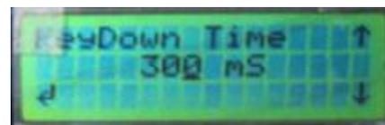
Different radio types have different 'Key down' times. This menu allows you to alter the time the Kestrel Control waits after sending last pack before trying to do anything else on the radio.
