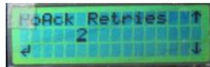
This menu defines the number of times the Kestrel Control transmits a data packet over the radio without an acknowledgement from the Master Kestrel before expiring the message.
