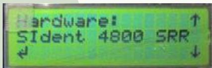
This menu selects what hardware is connected to device. SPORTident operates at either 4800 or 34000 baud rate. When either of the two SRR options are selected, the two SRR channels become ports 2 and 3, and the SRR module LEDs flash red.
