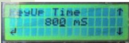
Different radio types have different 'key up' times. This menu allows you to alter the time the Kestrel Control waits to ensure the radio is fully powered up before transmitting the data.
